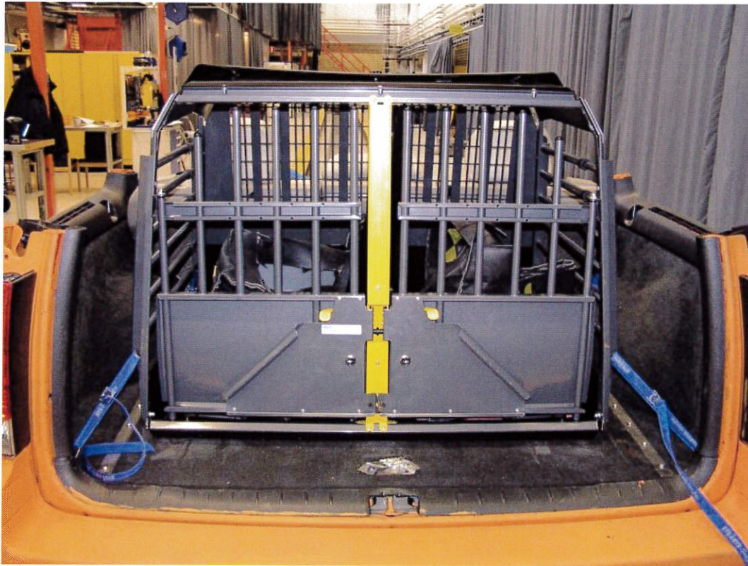
05 – After test, rear impact
