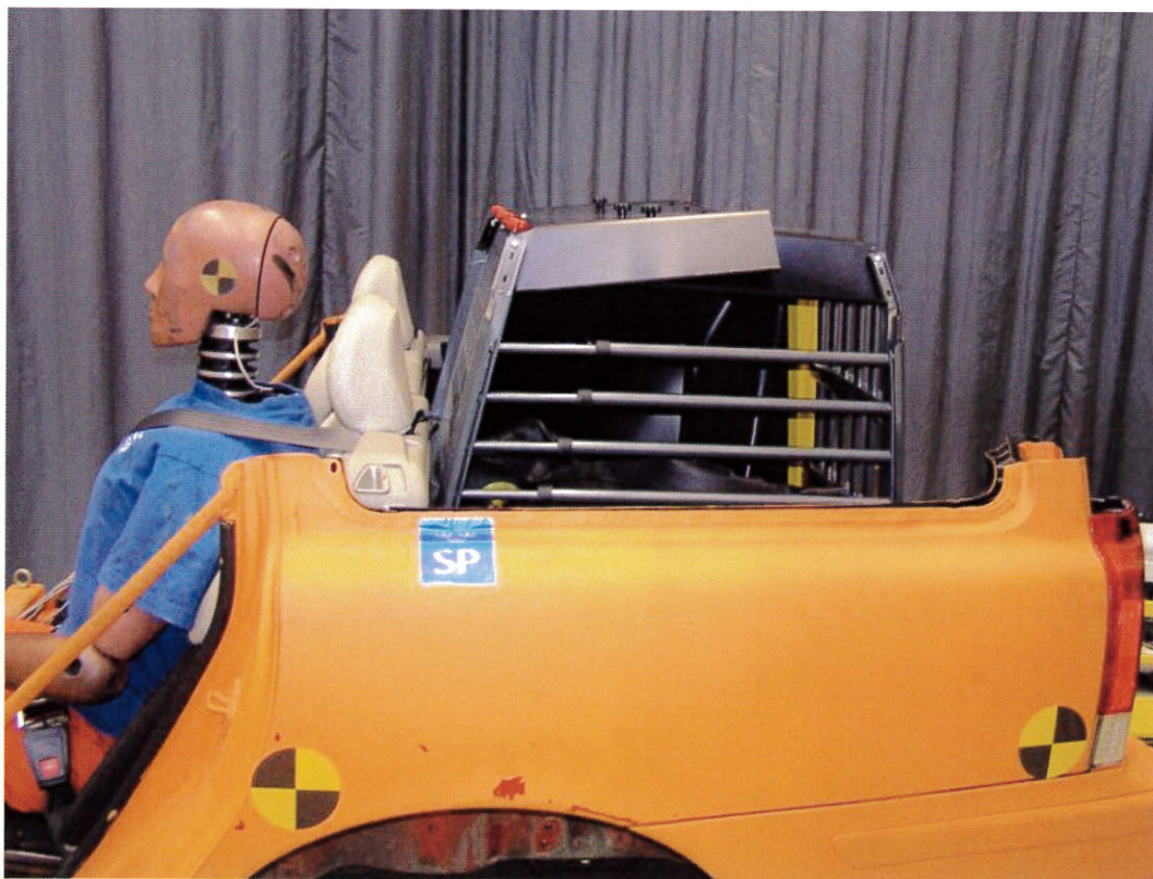
04 – After test, rear impact
