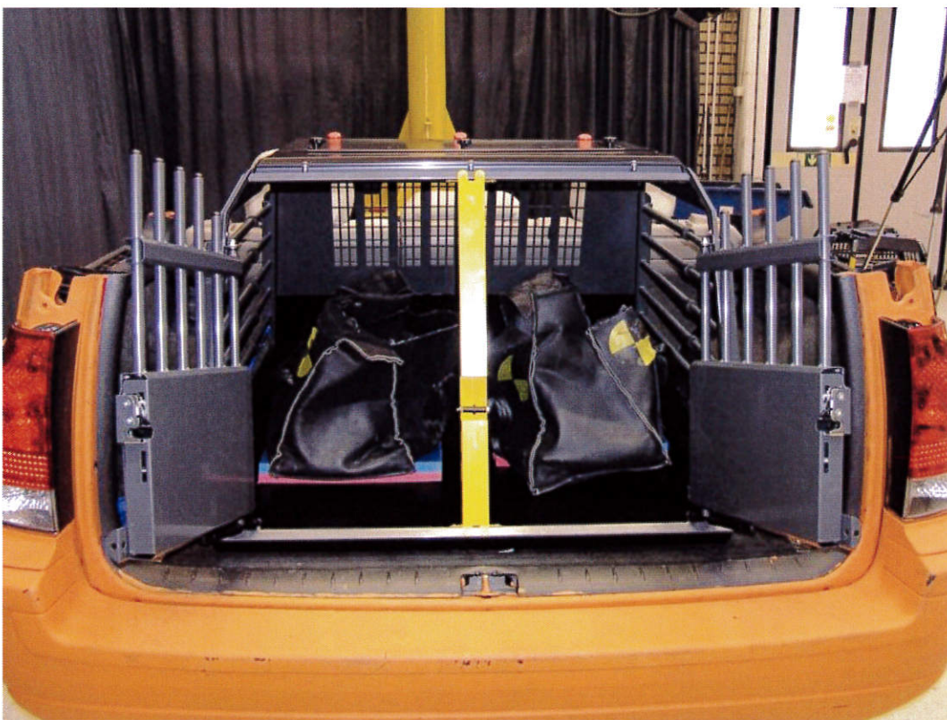
02 – Before test, frontal impact
