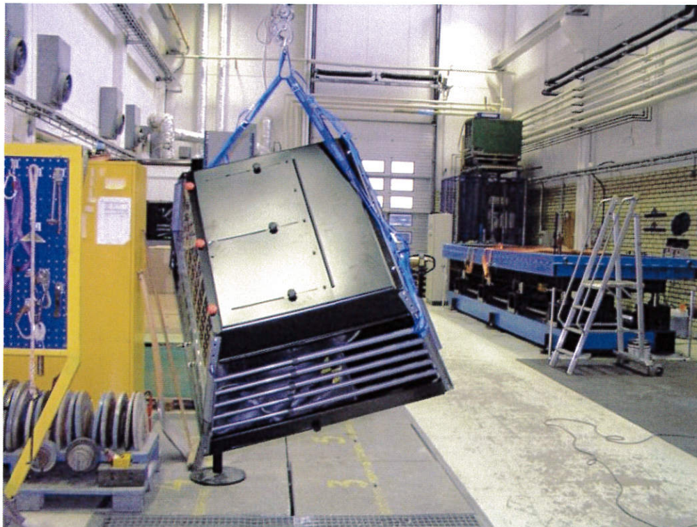
Figure 3 Test setup Drop test
